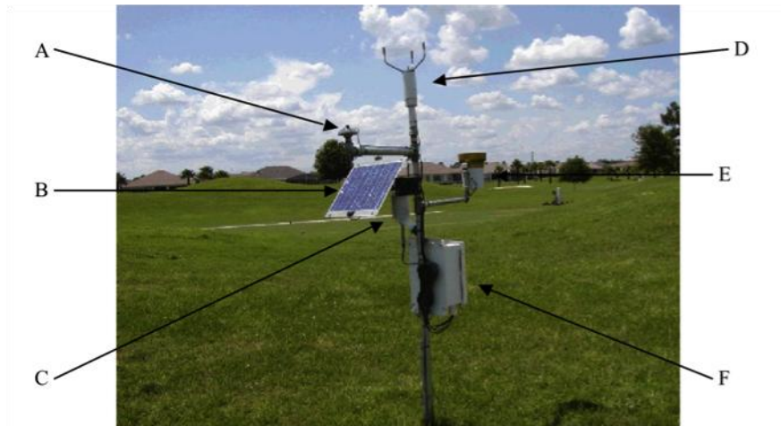
Figure 2.12. Anatomy of a weather station: (A) solar radiation sensor, (B) solar panel to power the station, (C) relative humidity sensor, (D) sonic anemometer to measure wind speed and direction, (E) tipping bucket to determine rainfall amount and duration, (F) datalogger enclosure.
